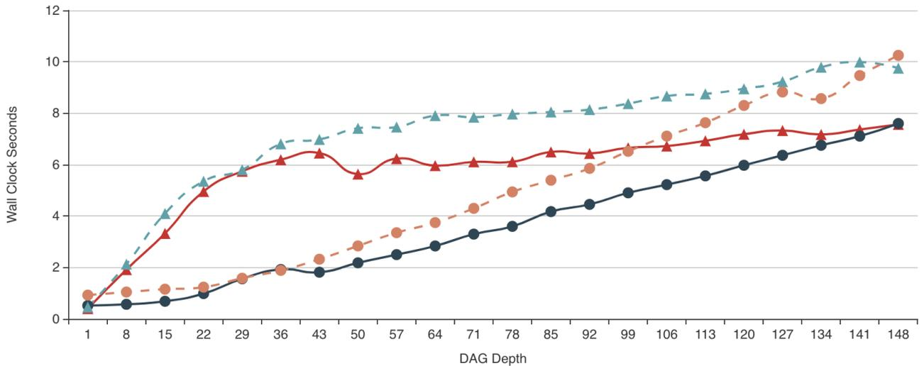
Immediately we can see that the non-modular builds roughly half in clock time matching the doubling of the available parallelism. And are now very close to the performance of GCC modular builds. What is striking is that the modular builds don't substantially change from the 8 parallel job case. And while before modular builds were faster at all depths now the non-modular builds have caught up at the highest depth of this test.
