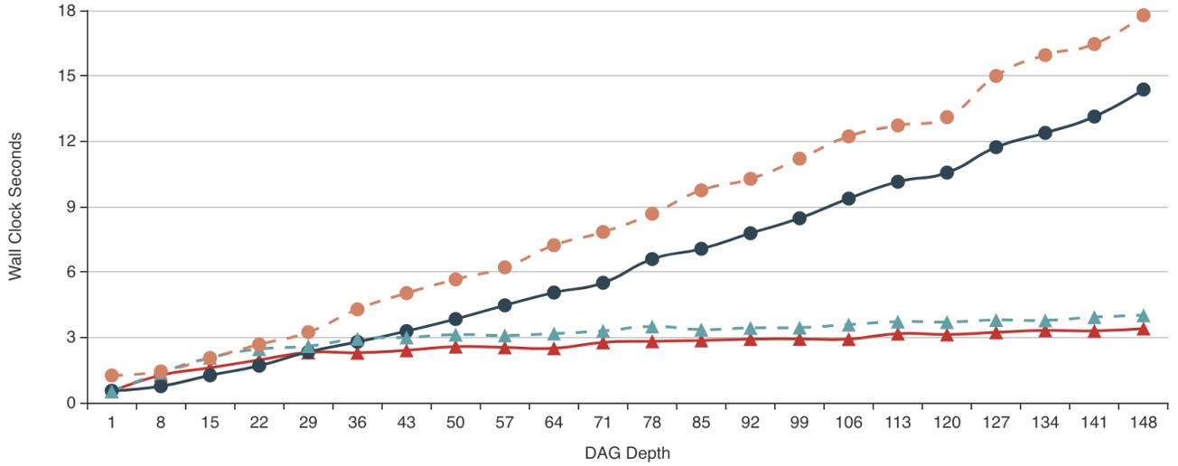
We've now reached the point where non-modular builds are faster at most DAG depths. And while the modular builds have stayed the same in the face of increasing parallelism, the non-modular builds have gained ground at each step.
