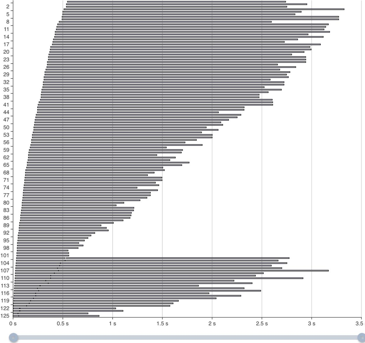
We can now see how the modular builds delay the execution of tasks as the dependency chain grows longer.
