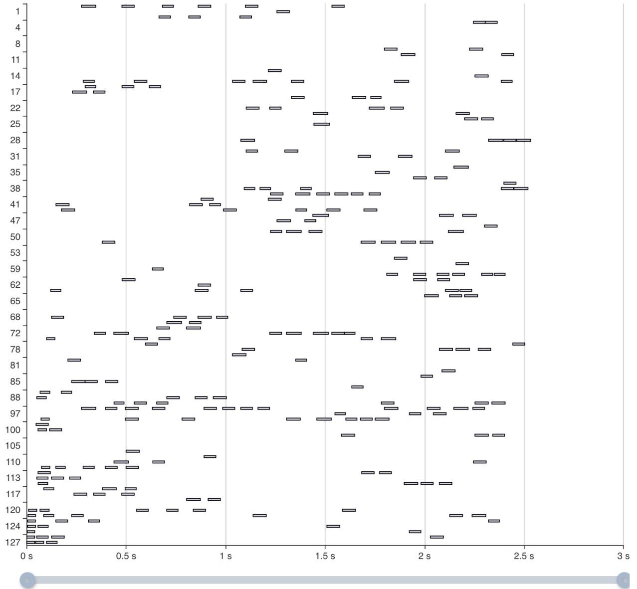
We can see above one key observation, there is a lot of unused CPU time during the overall build execution. This would be due to tasks needing to wait for the needed dependent tasks to complete. Below is the equivalent non-modular build.
