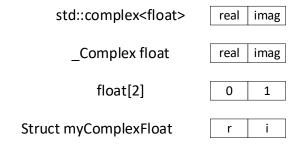
When many complex values are stored together, such as in a C-style array, a C++ std::array or a C++ std::vector, then the real and imaginary elements end up being interleaved in memory:
